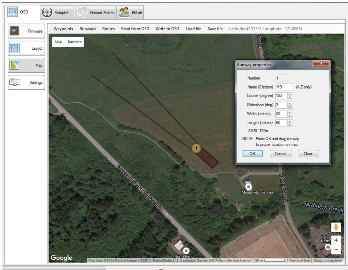
Figure 1 – Using the FPV Manager application to define a runway.
